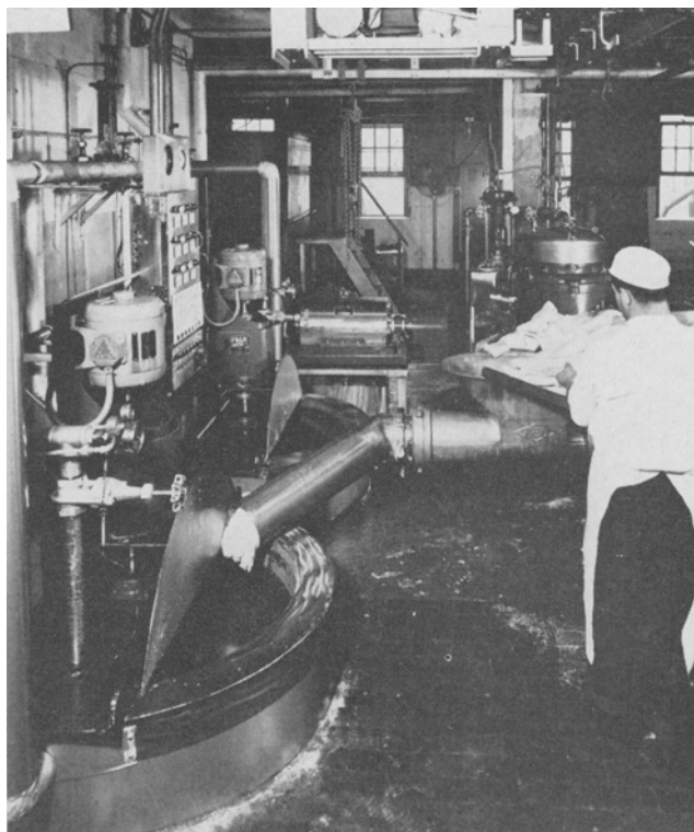
FIG. 2. Ground fat is fed to jacketed heating tanks. Sharples Super-D-Canter and Autojector are shown in the background.
